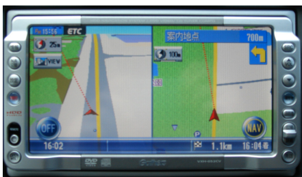
Fig. 2. An example of a commercially available car navigation system. A 3D perspective view of a road network (left) and its corresponding bird's-eye-view (right).
