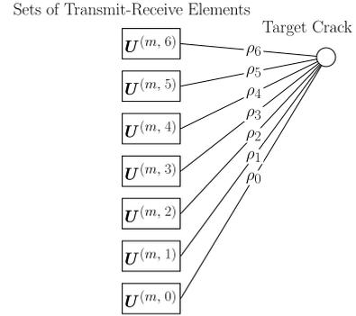
Fig. 3 Geometric relation between the transmit-receive elements and the focal point.
