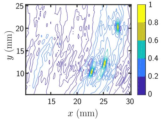
Fig. 5 Image constructed by using the proposed sequence set with a sensor array.
