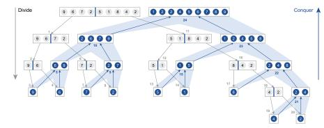
The operation of Merge Sort on the array  $A = \{9, 6, 7, 2, 5, 1, 8, 4, 2\}$ . The lengths of the sorted sequences being merged increase as the algorithm progresses from bottom to top.
