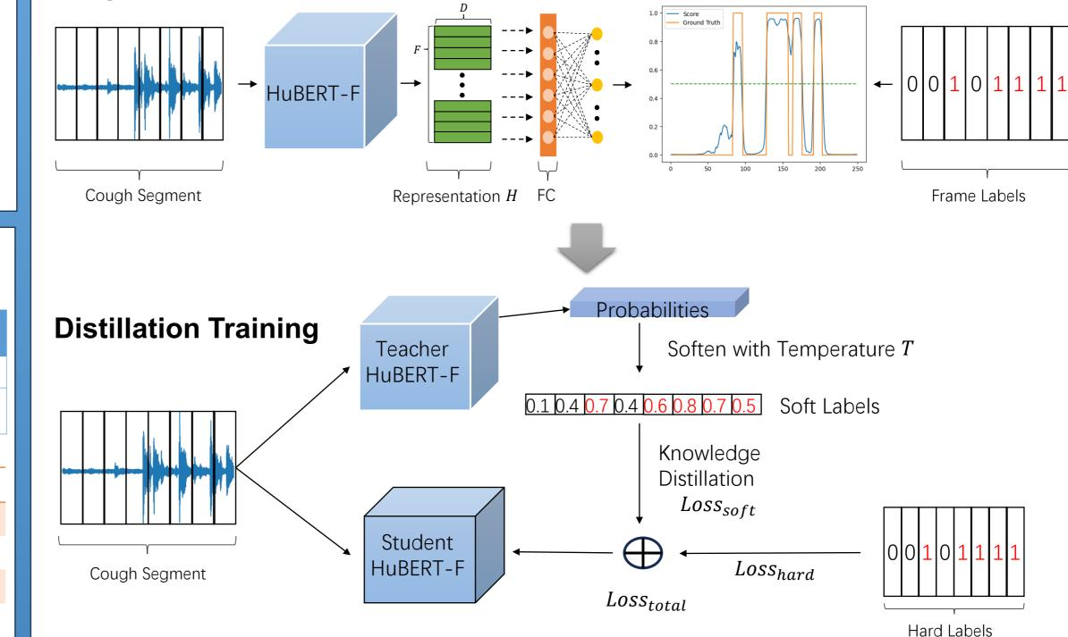
The performance of HuBERT-F increases, if the learning process is guided by a probability-distribution-like labels i.e., the soft labels, instead from hard coded zeros and ones i.e., the hard labels. Therefore, the knowledge distillation training is applied here aiming to generate the soft labels.
