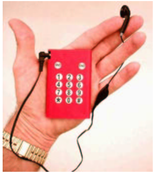
Fig. 9: Dieceland Technology disposable mobile phone. 43 This 2” × 3” (the size of a thick credit card) disposable ($10) mobile phone is made by printing cell-phone circuitry onto a paper substrate, which is then laminated.
