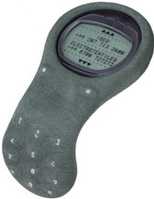
Fig. 8: ElekTex soft cell phone, 34 with touch controls integrated into the fabric. (©ElekSen. Photo by Marcus Rose.)
