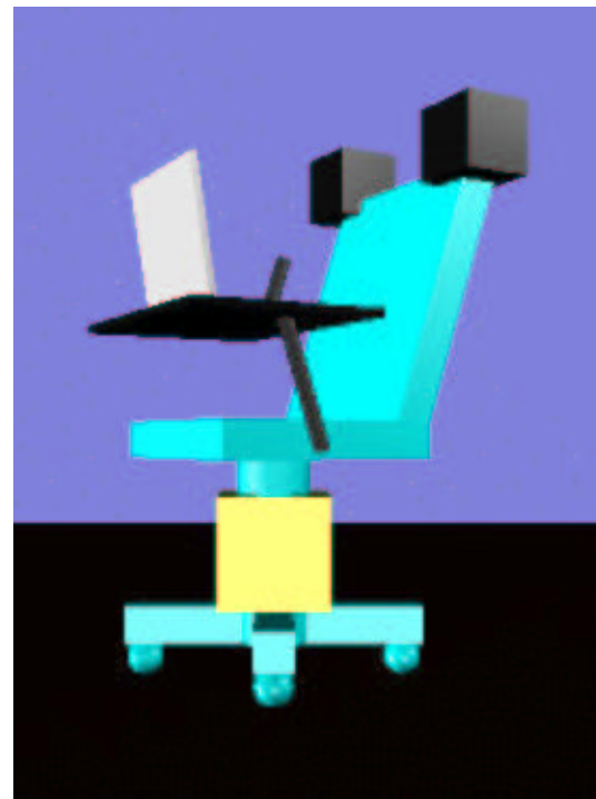
Fig. 16: Internet Chair with servomotor rotation: a pivot (swivel, rotating) chair deployed as an I/O device, an information appliance. The input modality is orientation tracking, which can dynamically select transfer functions used to spatialize audio in a rotation-invariant soundscape. In groupware situations, like teleconferencing or chat spaces, such orientation tracking can also be used to twist iconic representations of a seated user, avatars in a virtual world, enabling social situation awareness via coupled visual displays, soundscape-stabilized virtual source locations, and direction-dependent projection of non-omnidirectional sources. As an audio output modality, transaural speakers, nearphones in the headrest, can present unencumbered binaural sound with soundscape stabilization for multi-channel sound image localization. As a haptic output modality, servomotors will render kinesthetic force-feedback, turning each chaire (pronounced “ schaire ,” for “share-chair”) under networked control, distributing torque across the internet to direct the attention seated subjects (with adjustable insistence/forcefulness), orienting seated users (like a “dark ride” amusement park attraction), or subtly nudging them in a particular direction. (Java3D model by Daisuke Kaneko.)
