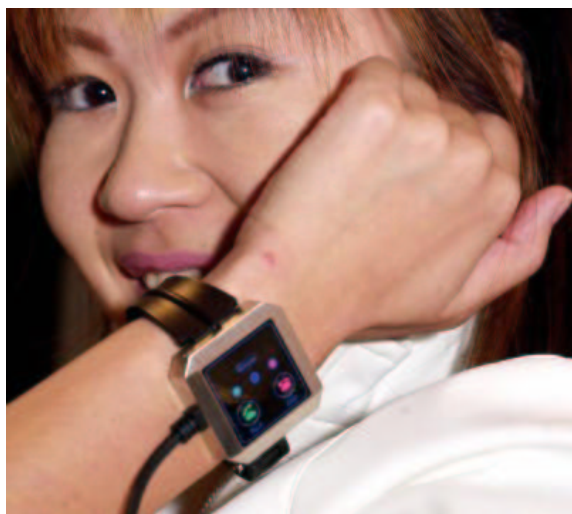
Fig. 13: NTT DoCoMo “Whisper Wearable Terminal.” By sticking her finger in her ear, a user can hear sound conducted through arm, hand, and finger bones while speaking into a microphone on the back of the wristband, snapping fingers to signal “connect” and “disconnect” commands. The manufacturer hopes to release a commercial model in 2005. Presumably a stereotelephonic system could be realized by sticking fingers in both ears.
