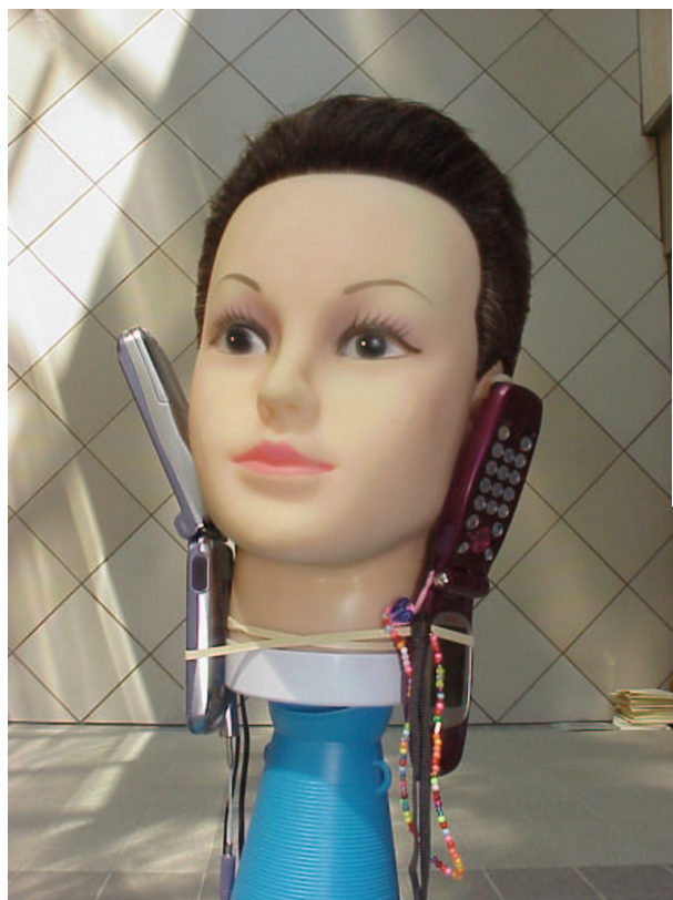
Fig. 6: “Poor person’s mobile stereotelephony”: a pair of inverted mobile phones, deployed as a microphone array attached to a dummy head, simultaneously calling a dual voice line (like an ISDN service) realizes wireless (if low-fidelity) binaural telepresence.
