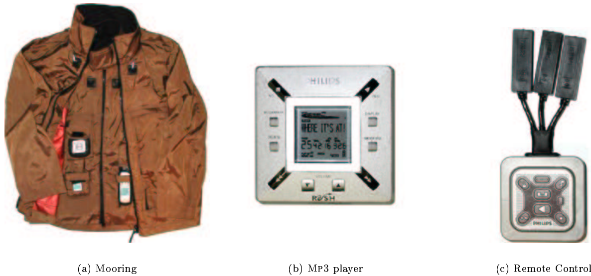
Fig. 11: Phillips and Levi-Strauss have teamed up to develop jackets with built-in electronic equipment, including an MP3 player, headset, mobile phone handset, and remote control. The system is equipped with a so-called “Personal Area Network,” or PAN, an electronic bus woven into jacket that allows transport of data, power, and control signals within the garment.
