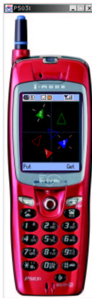
Fig. 3: NTT DoCoMo i-mode iappli iJade emulator running “ ι -Con” application. The quasi-realtime synchronization with CVE server motivates the use of “ghost icons” to distinguish local and session states of avatars. (Developed by Yutaka Nagashima and Makoto Kawaguchi.)
