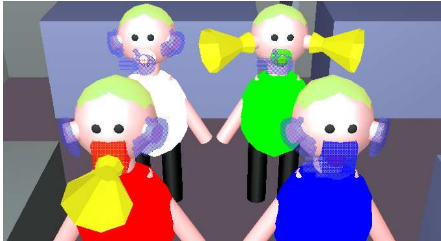
Fig. 7 Include narrowcasting operations in Multiplicity: The avatar in the front left is selected, so its complement (comprising all the other avatars) is muted (denoted by the translucent hands before the mouths), and the avatar in the back right is attended, so its complement is deafened (denoted by translucent hands before the mouth).
