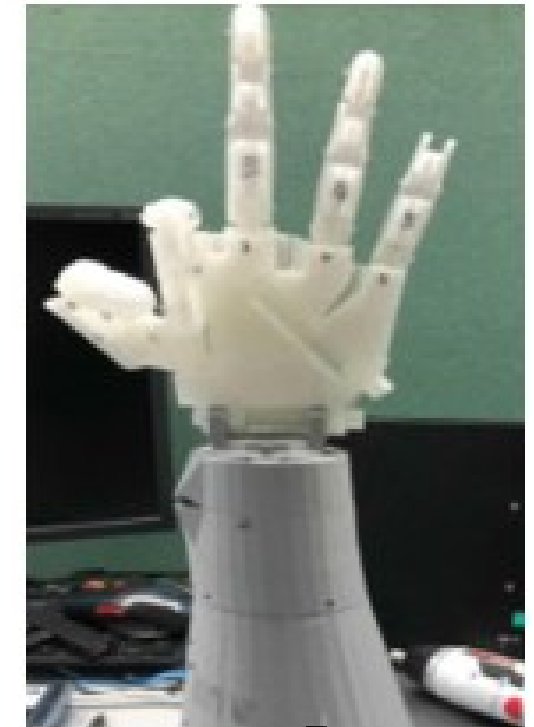
(b) AlzuHand: AlzuHand is a 3D-printed, low-cost prosthetic hand designed for EMG-based control with real-time feedback, a neuromorphic prosthetic hand with sensory-motor
