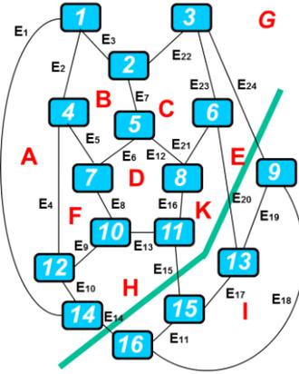
Fig. 4. A cut-set line based on the **E-K-H**-face path
