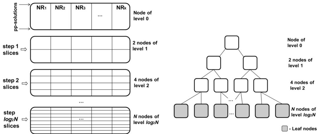
Fig. 15. Two views of the subproblem nodes in scheme 1
