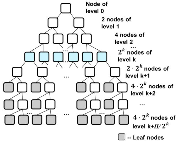
**Fig. 17. Subproblem nodes in a combination of schemes 1 and 2**
